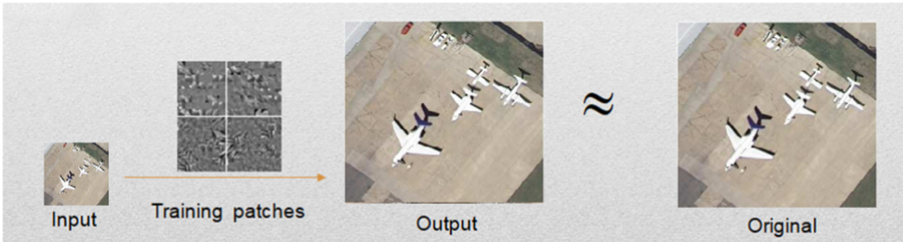
Fig. 5. Sparse coding for super-resolution reconstruction
