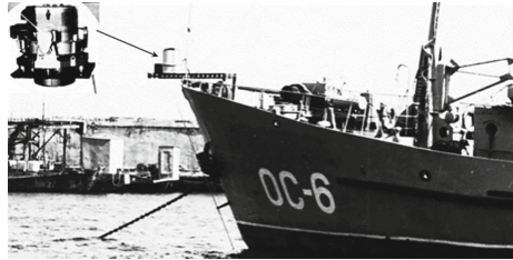
Fig. 10. A ship with an installed thermal imager
