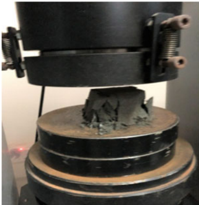
(c) Compressive strength testing of mortar cube samples
