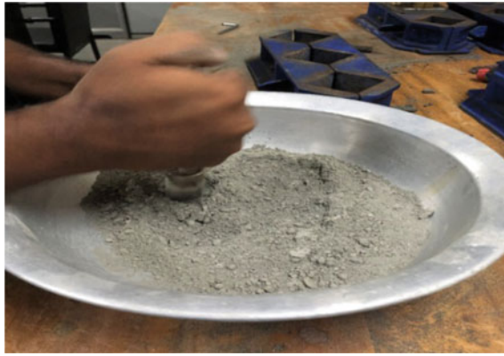
Fig. 3 Crushing of oven dry sludge to make it powder
