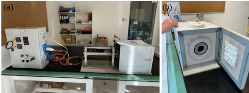
Fig. 3 Picture of a mini rotary kiln with control panel and b front view
