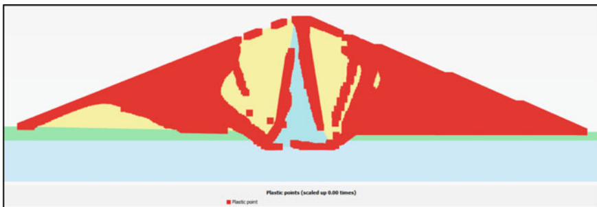
Fig. 9 Distribution of plastic points over the dam section in FEM pseudo-static analysis
