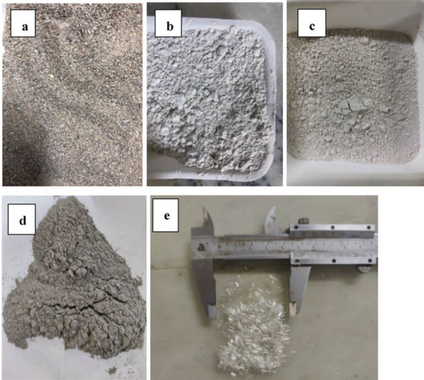
Fig. 2 Materials used in the study. a Sand, b Ca-Bentonite, c Colemanite, d Copper slag, e Glass fiber
