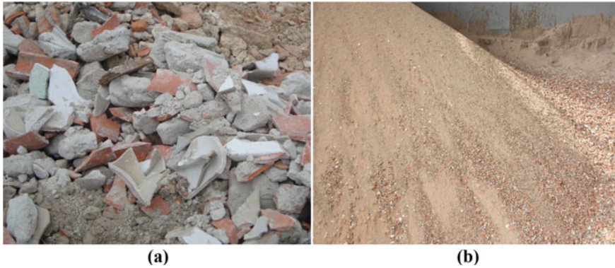
Fig. 1 Visual appearance of: a the C&D waste at the recycling plant; b fine-grain recycled C&D material
