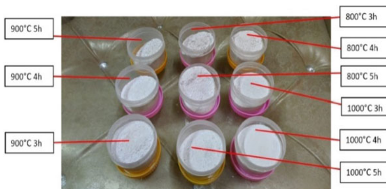
Fig. 2 Snail shell calcinated at a temperature of 800, 900, and 1000 °C and time of 3, 4, and 5 h
