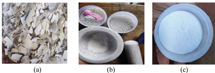
Fig. 1 Preparation of CaO catalyst
