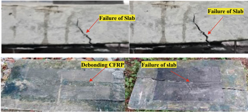
Fig. 10 Failure mode without CFRP attached slab and with CFRP attached slab
