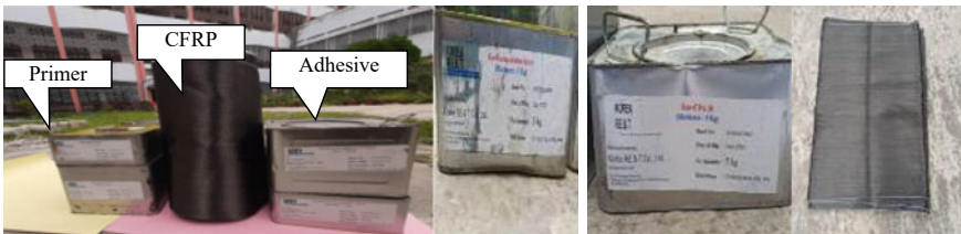
Fig. 1 Primer, CFRP fabric, and adhesive
