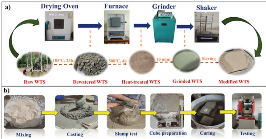
Fig. 1 a Schematic diagram for the preparation of modified WTPS, b Schematic diagram for step by step procedure for concrete casting and testing
