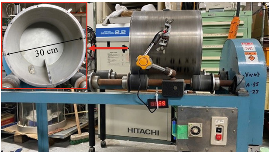
Fig. 4 Rotary drum abrasion test setup
