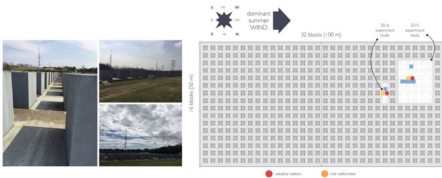
Fig. 1 Footage and plan view of the overall experimental study at the COSMO (Syafii et al., 2017a)
