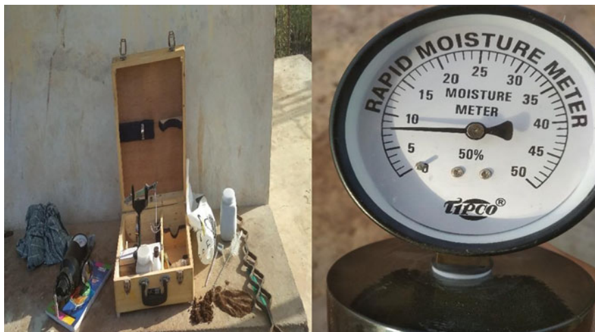
Fig. 2 Rapid moisture meter to measure water moisture in soil
