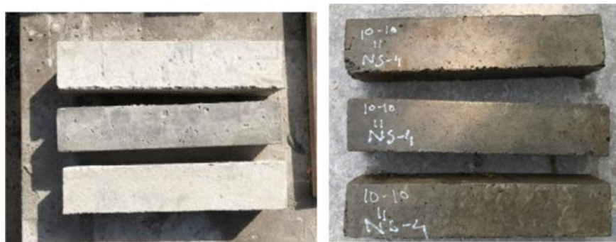
Fig. 4 Control and 3% nano-silica beams for flexure
