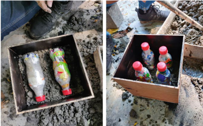
Fig. 8 Ecobrick in mortar mould
