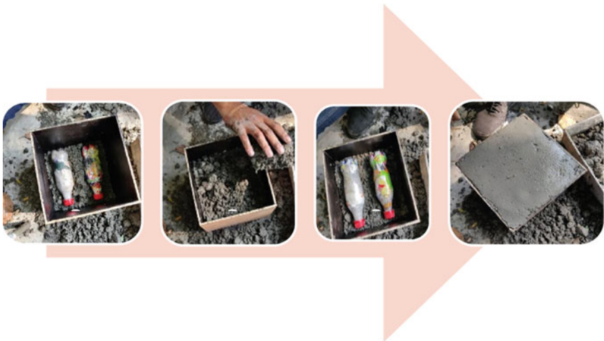
Fig. 9 Process of cubical mould formation
