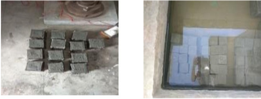
Fig. 2 Casting and curing of cement mortar cube
