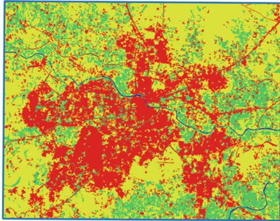
Fig. 6 Manual edits applied over the (3 × 8) sieved maximum classified LC map to develop the final LC map for the Nashik region
