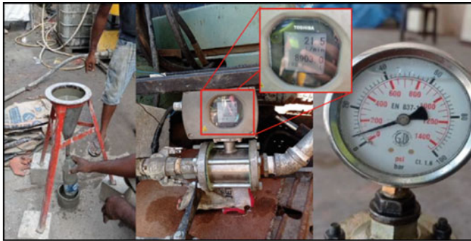
Fig. 12 Flow cone test, flow Meter, and pressure gauge
