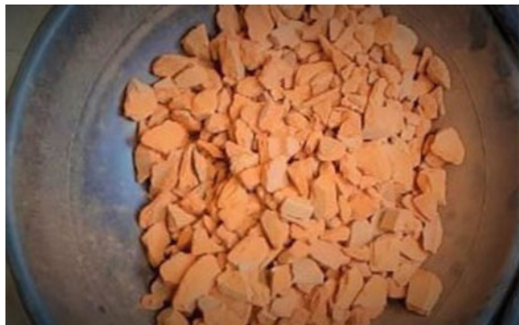
Fig. 7 Mechanically crushed waste Calicut tiles
