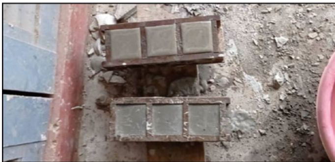
Fig. 13 Casting of grout test cubes
