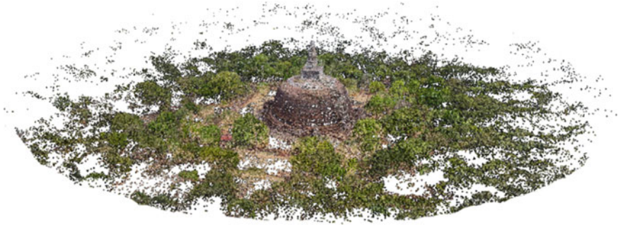
Fig. 7 3D point cloud of Rankoth Wehera generated using Meshroom software
