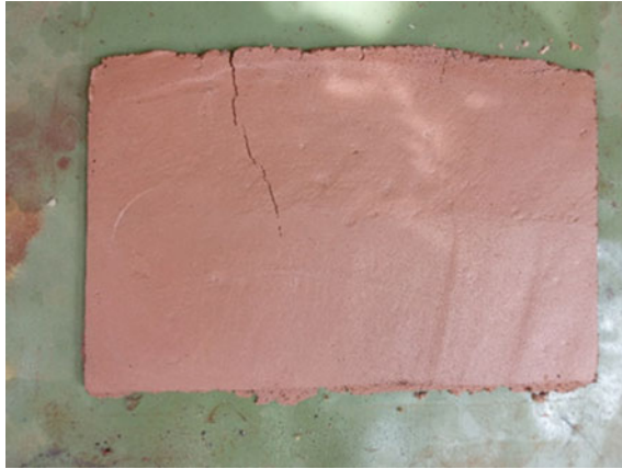
Fig. 2 A Non-reinforcement wall panel composed of cement and soil
