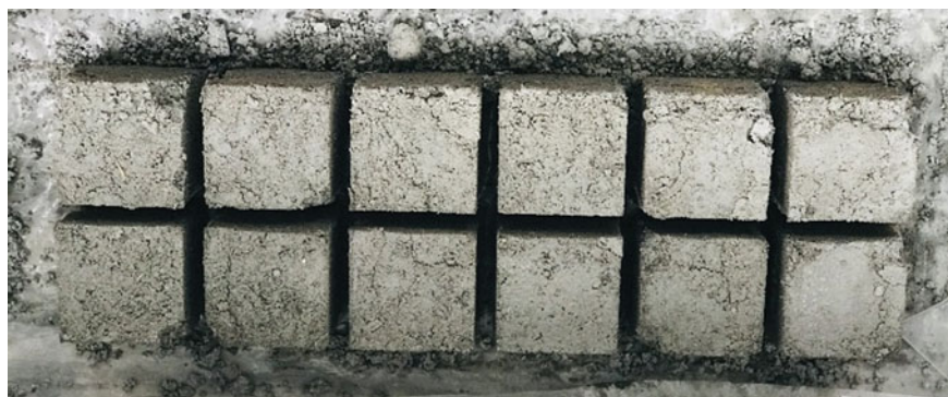
Fig. 3 Cement blocks after removing the mold
