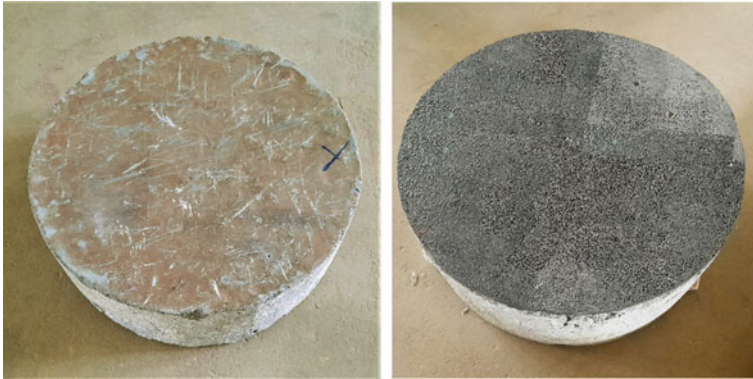
Fig. 3 Prepared concrete sleeper (left) and recycled USP attached to the concrete sleeper (right)
