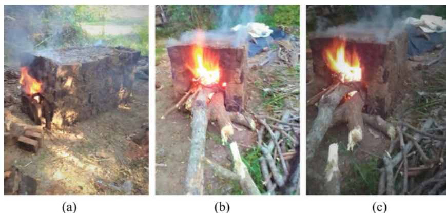
Fig. 2 Firing process: a the initial state of the firing of aggregates, b after 2 h—start the firing process, c after 4 h—starting the firing process
