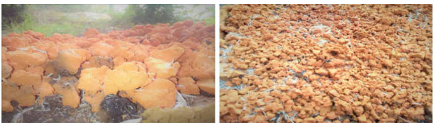
Fig. 5 Aggregates derived from the water treatment plant's sludge
