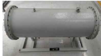
Fig. 3 Platform of DC GIS metal particle motion and discharge characteristics testing
