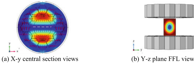
Fig. 3 FFL generated by permanent magnet array
