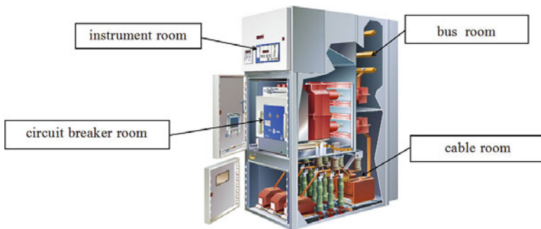
Fig. 3 Intelligent high voltage switchgear diagram
