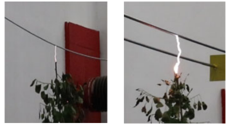
(a) 110kV breakdown arc (b) 220kV breakdown arc
