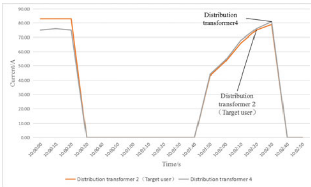
Fig. 6 Current curve of standby supply path 2
