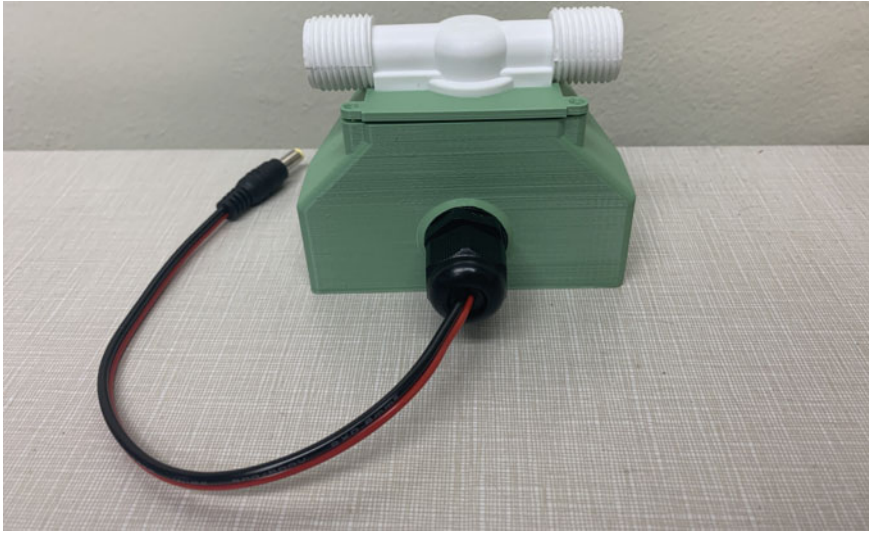
Fig. 8 Solenoid valve in 3D-printed case
