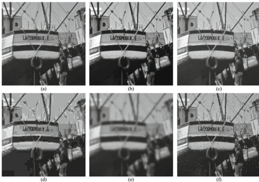
Fig. 3 Comparison of degradation of the ship image [15] with different degradation levels. All images have a L_1 loss value of 15. a Original image; b MSSSIM = 0.9168; c MSSSIM = 0.9900; d MSSSIM = 0.6949; e MSSSIM = 0.7052; f MSSSIM = 0.7748
