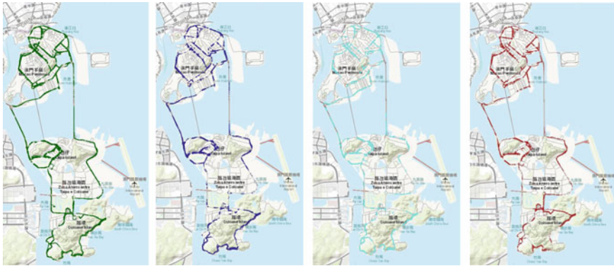
Fig. 3 Heatmap of four carriers. Traverse all points of the drive test. If the four indicators of a point RSRQ, CINR, RSSI, and RSRP are excellent, the point is drawn on the map by latitude and longitude. Left to right are Carrier A, B, C, and D
