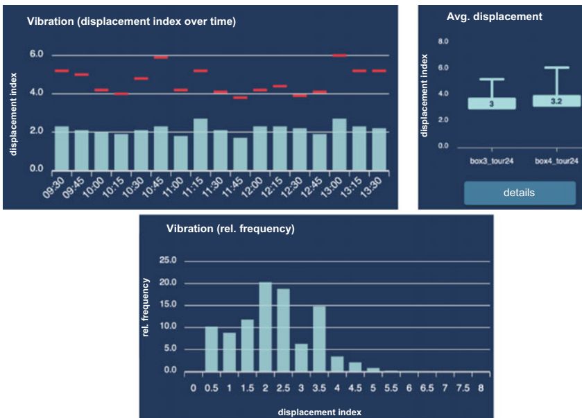
Fig. 9 Implemented diagrams to display the vibration as displacement. Top Left: A bar chart was extended with horizontal lines above the bars to show the maxima. Top right: A modified box plot to show max and average displacement. Bottom: A histogram to show the relative frequencies of displacement
