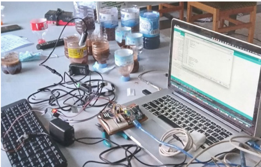
Fig. 2 Measuring soil parameters using Arduino ATMEGA 2560 R3
