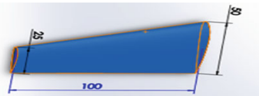
Fig. 11 NACA2411 airfoil (max thickness-11% at 29.5% of chord and max camber-2.5% at 39.6% of chord)
