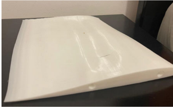
Fig. 7 Warping of the wing material used PLA
