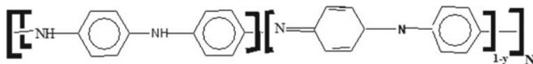
Fig. 6 Three stable forms of PANI are in correspondence to the values y = 0 (leucoemeraldine base, LB), y = 0.5 (emeraldine base, EB), and y = 1 (pernigraniline base, PNB). Where y gives the average oxidation degree
