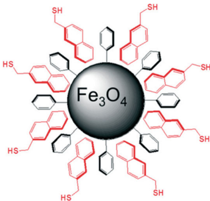
Fig. 4 Schematic diagram of non-covalently functionalized \text{Fe}_3\text{O}_4 nanoparticles. The phenyl ligand shell (in black) helps non-covalent interaction with the thiol bearing layer. Reproduced with permission from Ref. [18]. Copyright 2015, Royal Society of Chemistry
