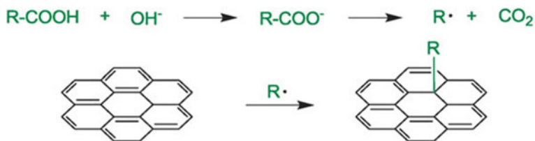
Fig. 10 Free radical addition of radical species onto graphene (bottom) and Kolbe reaction toward the formation of radical species (top). Reprinted with permission from The Royal Society of Chemistry 2013 and Ref. [97],
