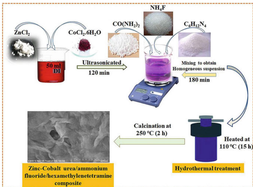
Fig. 4 Schematic illustration of the ZC-UAH composite preparation process by a facile hydrothermal process. "Reprinted (adapted) with permission from [45] Copyright (2020) Elsevier"
