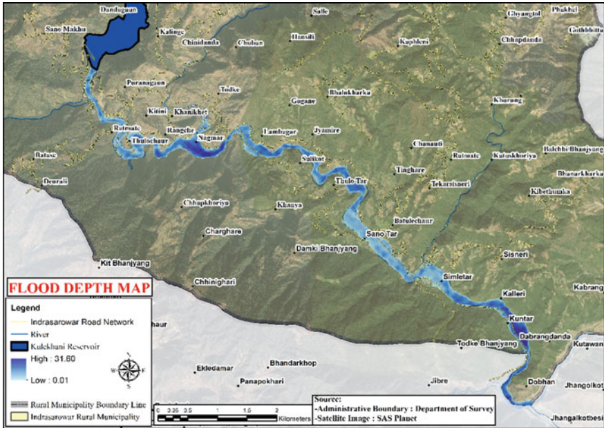
Fig. 6 Flood hazard mapping of dam outbreak (Source flood hazard analysis)
