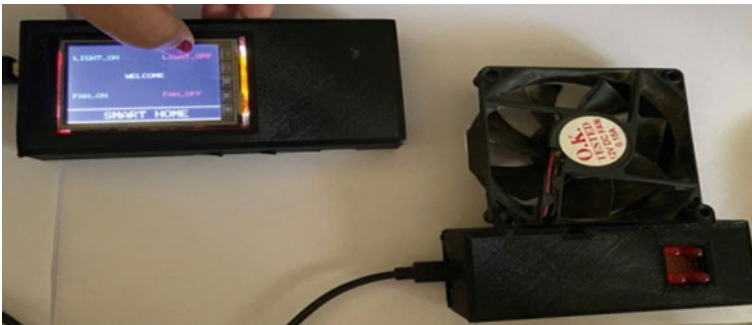
Fig. 8 When we press the LIGHT-OFF button, it stops glowing and the lights switch off
