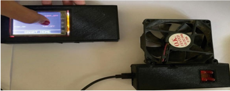
Fig. 10 When we press the FAN-OFF button on the touch control panel, the fan goes off
