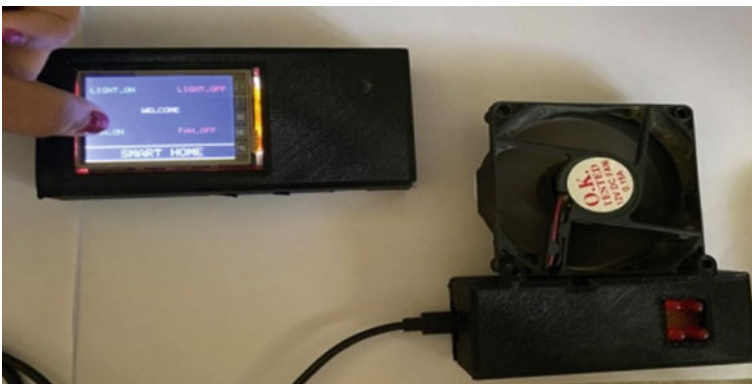
Fig. 9 When we press the FAN-ON button on the touch control panel, the fan turns on
