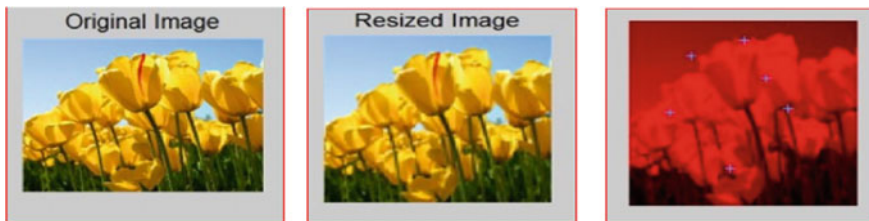
Fig. 1 An selected Image (Is) which is resized to particular dimensions referred as resized Image. Later this resized image undergoes conversion process resulting to red channel Image (Ir). This red channel image is used for mouse pointed points by the end user as shown above
