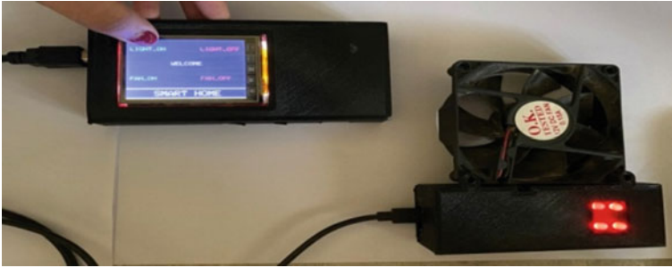
Fig. 7 When we press the LIGHT-ON button on the touch control panel, led light bulbs turn on
