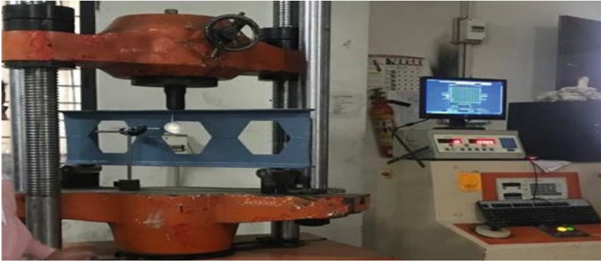
Fig. 5 A figure shows experimental test set up for testing of castellated beams
