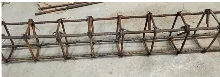
Fig. 1 Reinforcement details of Beam 1
