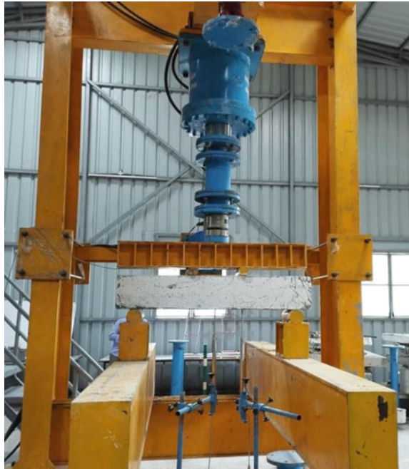
Fig. 5 Loading frame with beam
