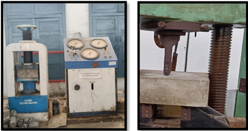
Fig. 5 Compressive and flexural test of paver block
