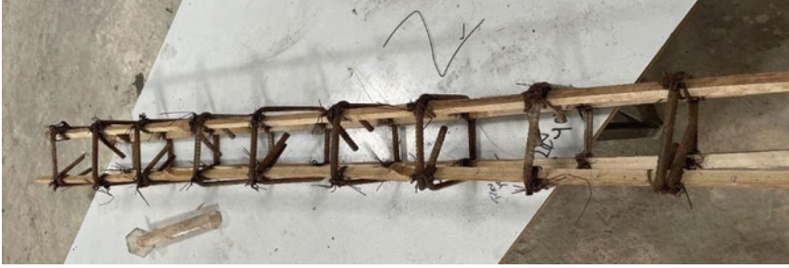
Fig. 3 Reinforcement details of Beam 3
