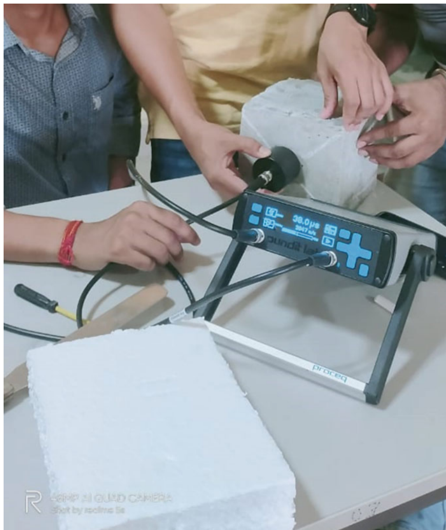
Fig. 7 Ultra pluse velocity test on M20 cube
