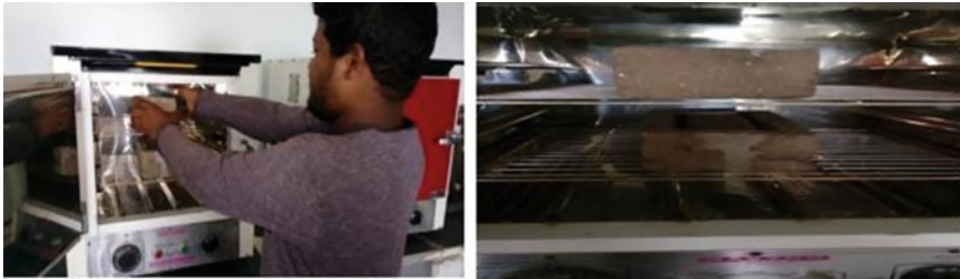
Fig. 4 Placing brick in the oven for drying
