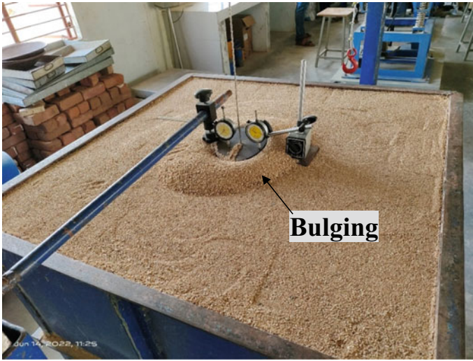
Fig. 3 A Photographic view of reinforced sand bed after failure
