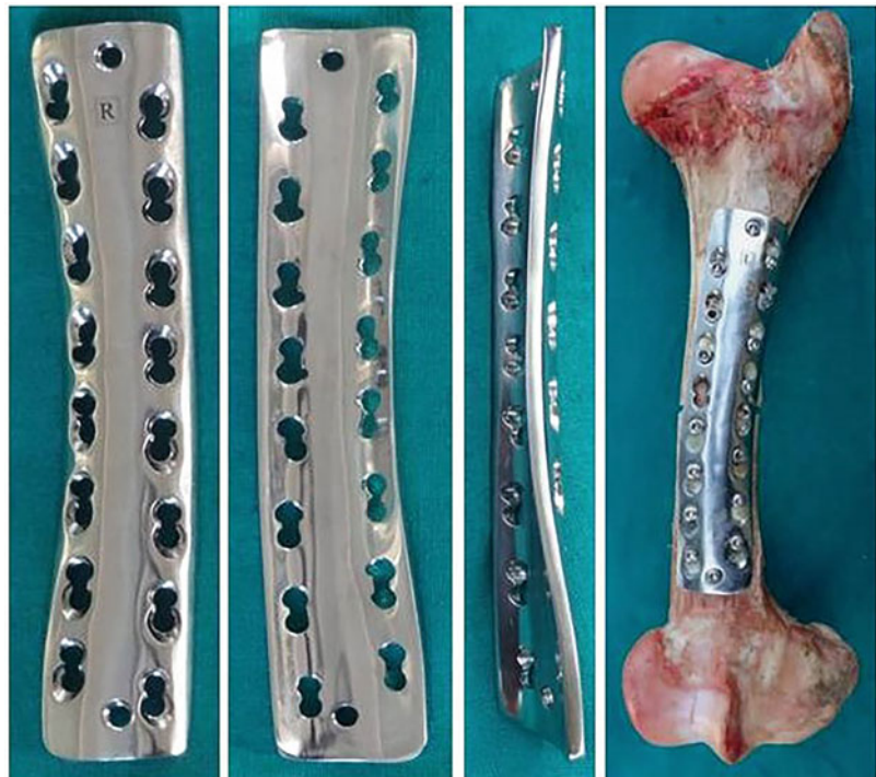
Fig. 2.39 Contoured locking compression plate developed for bovine femur
