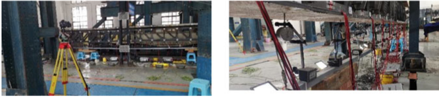
Fig. 4. Measuring Camera and Dial Indicator Arrangement
