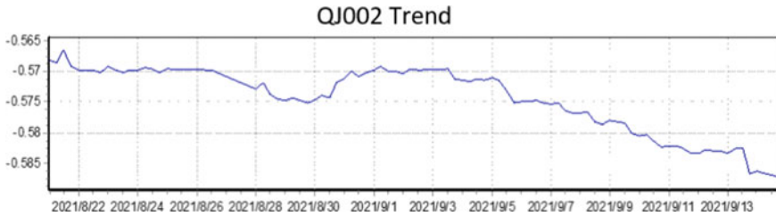
Fig. 5 Automatic tilt east side monitoring curve
