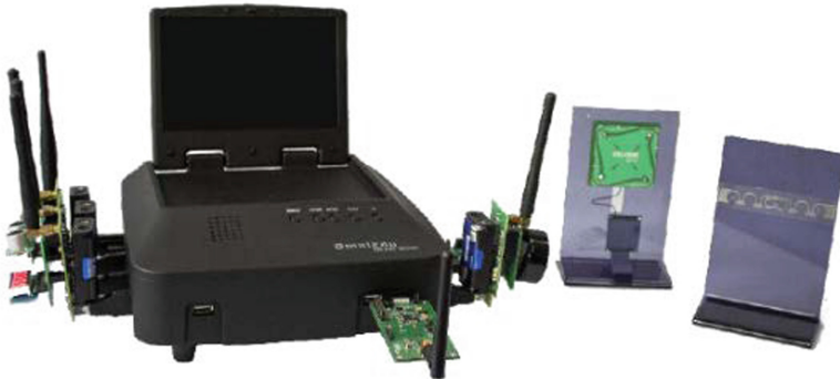
Fig. 3. Smart Node: An Embedded Node with Interfaces for Sensor Nodes.
