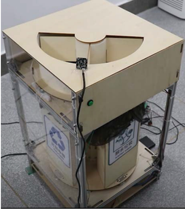
Fig. 5. Garbage sorting device made by students based on the course.
