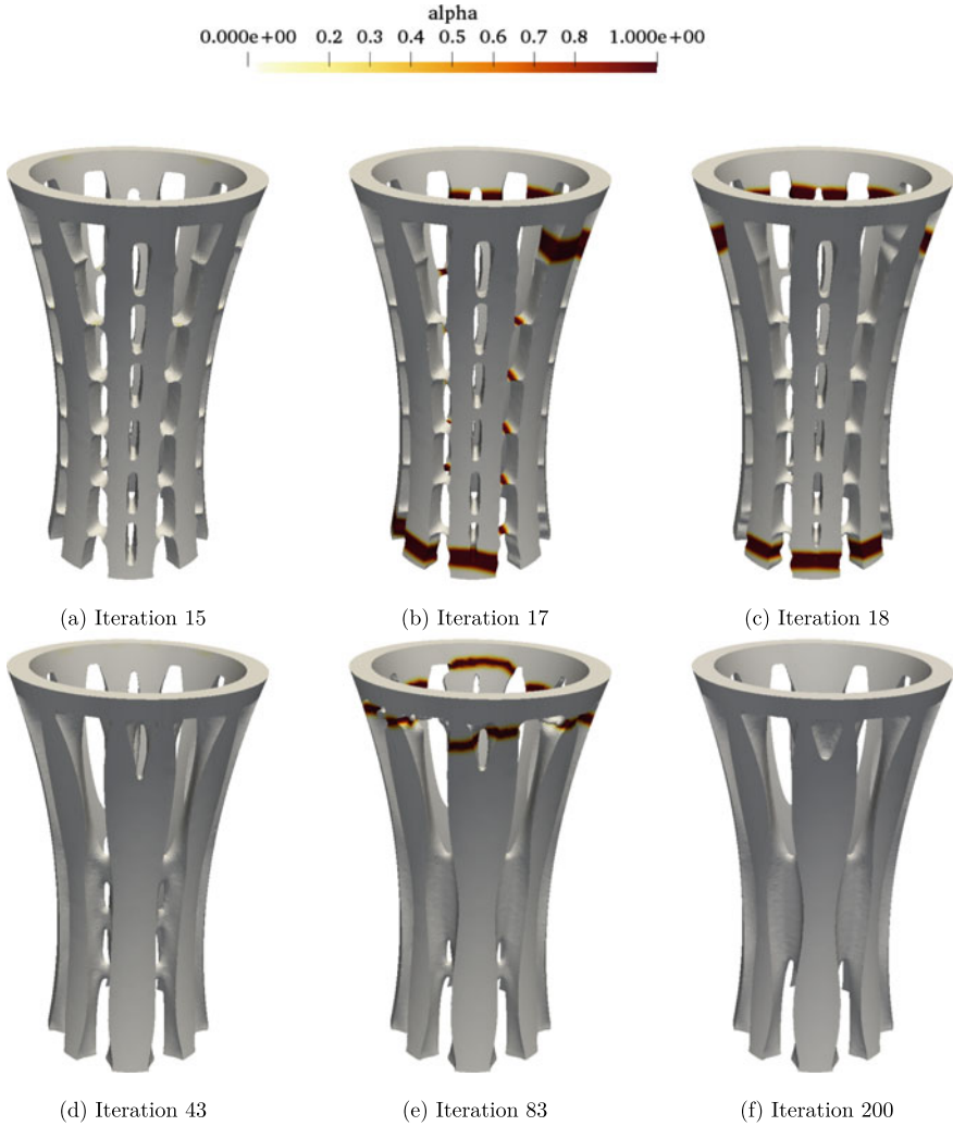
Fig. 8.48 Damage variable \alpha at the final time T plotted for several optimization iterations for the shape in Fig. 8.47 (black regions indicate cracks)
