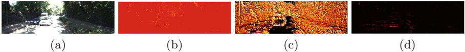
Fig. 1. Parametrization of the gradient covariance matrix using an urban image. (a) Color reference image. (b) scale \gamma_i , (c) orientation \theta_i and (d) dominant orientation \sigma_i .
