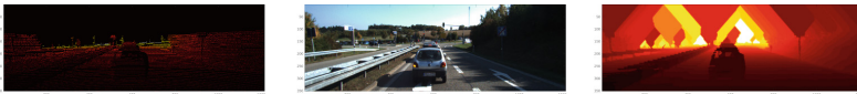
Fig. 5. Left image, sparse depth map. Center, color reference image. Right, completed depth.
