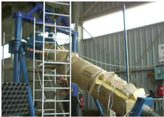
Fig. 4 Water tightness test setup
