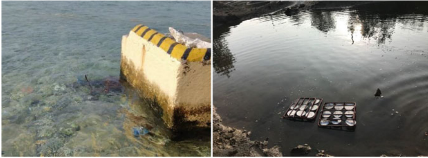
Fig. 5 Photos of immersed sampled in tides zones of Khanh Hoa region (left) and Ha Long Bay (right)
