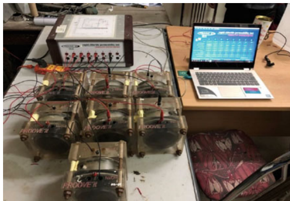
Fig. 3 Experimental set-up for chlorine ion penetration test in UTC Lab
