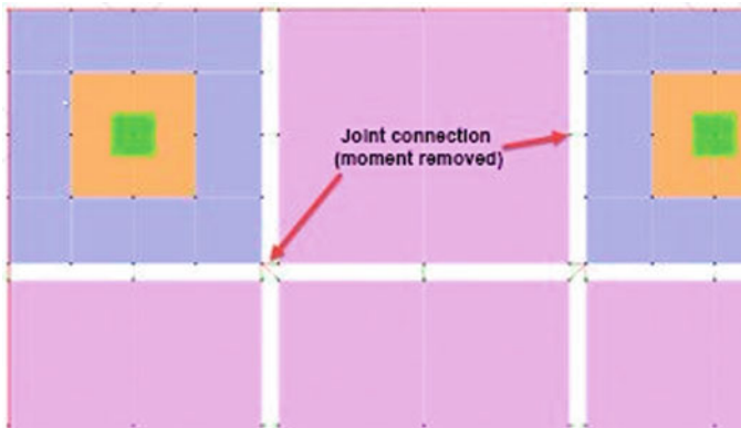
Fig. 6 Simulation of panels with joint connections
