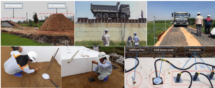
Fig. 2 Full-scale test of embankments and monitoring equipment at Ba Ria-Vung Tau province, Vietnam
