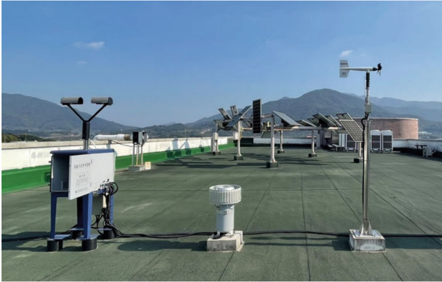
Fig. 1 Parsivel disdrometer located inside the Kyungpook National University campus
