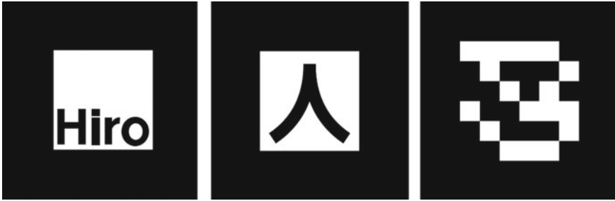
Fig. 6.1 Early examples of the augmented reality fiducial markers (left and center: ARToolkit and right: ARTag)
