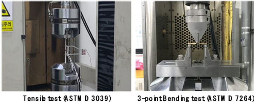
Fig. 6 Material property measurement tests
