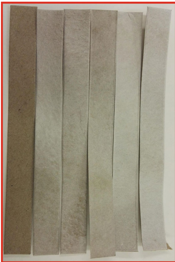
Fig. 17.49 Spray-coated nanocellulose barrier layers on the paper substrates
