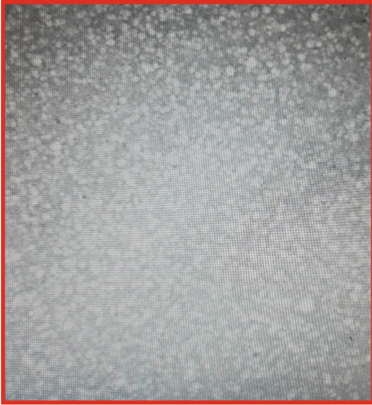
Fig. 17.28 Uniformity of spray-coated nanocellulose film
