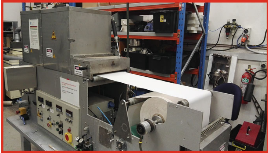
Fig. 17.50 Concept for continuous process for spray-coating nanocellulose on the paper substrates
