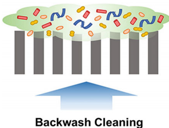
Fig. 15.3 Schematic of backwashing the membranes. Adapted with permission from Kim et al. (2018) Copyright (2018) American chemical society
