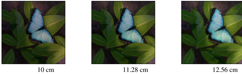
Fig. 12.8 The reconstructed images at each distance from the complex hologram calculated with the compensate phase
