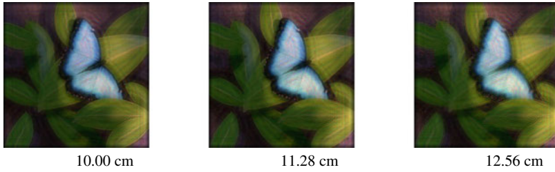
Fig. 12.4 The reconstructed images at each distance from the amplitude hologram calculated with the compensate phase
