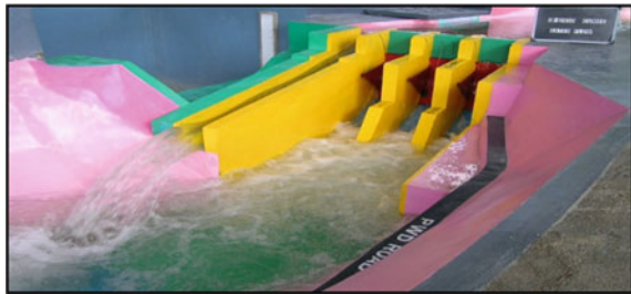
Photo 9 Performance of Energy dissipator of the chute spillway for Q = 4010 ( 2850 + 1160 ) m^3/s at FRL El 1397 m
