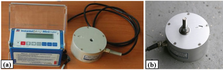
Fig. 6 A digital engineering seismograph (mini-mate, M/s InstanTel Inc., Canada)
