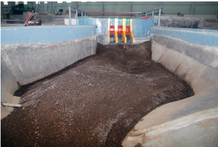
Fig. 7 Scoured river bed downstream of the spillway, Q = 5000 \text{ m}^3/\text{s} (100%), FRL El. 245.15 m
