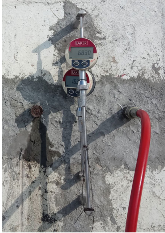
Photo 4 Fixing of four pins for determining in-situ Poisson's ratio
