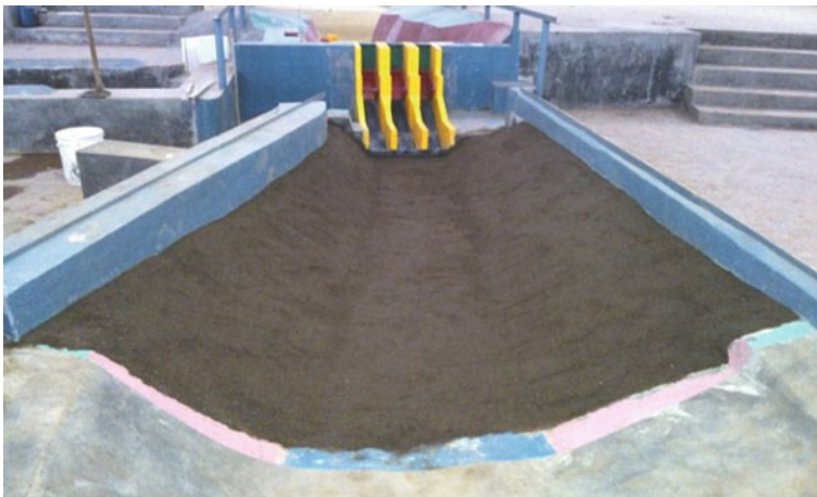
Fig. 5 Downstream view of the model showing reproduction of river portion with erodible material
