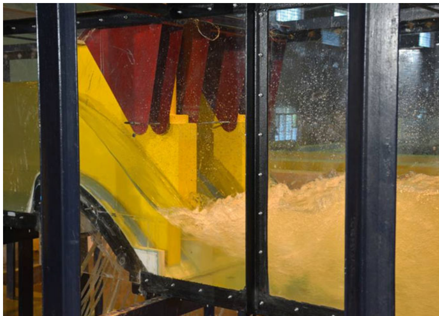
Photo 4 Flow condition on chute block and in stilling basin for design maximum discharge with gates fully open in modified design-I
