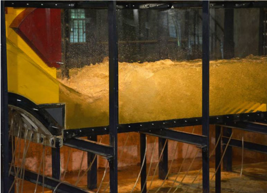
Photo 3 Flow condition on chute block and in stilling basin for design maximum discharge with gates fully open in original design
