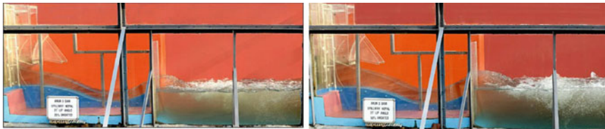
Fig. 10 Performance of energy dissipator for ungated operation of spillway
