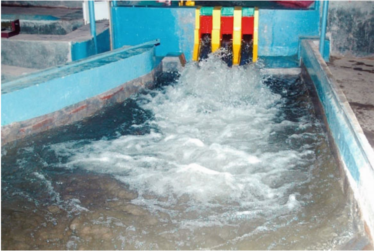
Fig. 6 Flow condition in the river downstream of the spillway, Q = 5000 \text{ m}^3/\text{s} (100%), FRL El. 245.15 m
