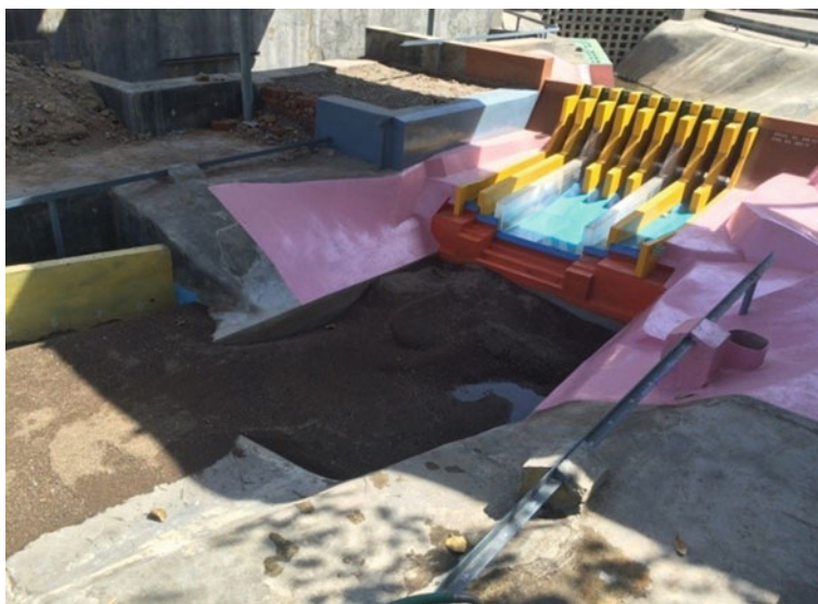
Fig. 13 Scour pattern for the design discharge of 50% of PMF with the gated operation of the spillway
