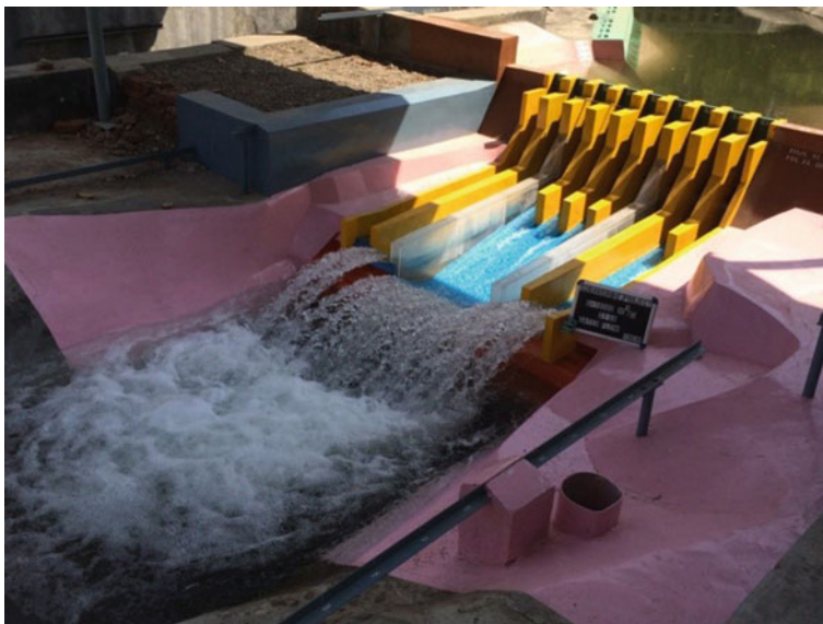
Fig. 12 Flow conditions downstream of the spillway
