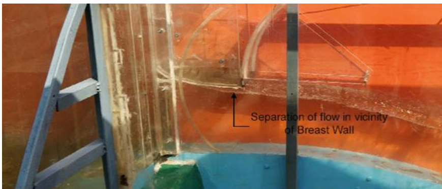
Fig. 4 Flow condition in the vicinity of breast wall bottom profile
