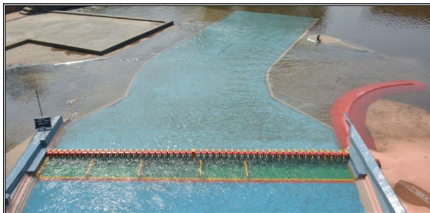
Fig. 3 Flow conditions in the approach channel and near the guide bund
