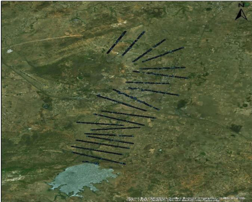
Fig. 3 River cross-sections on downstream of Umrar Dam
