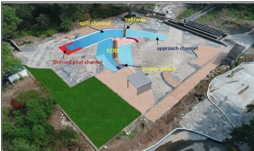
Fig. 2 Aerial view of 1:140 scale model of various components of Polavaram Irrigation project
