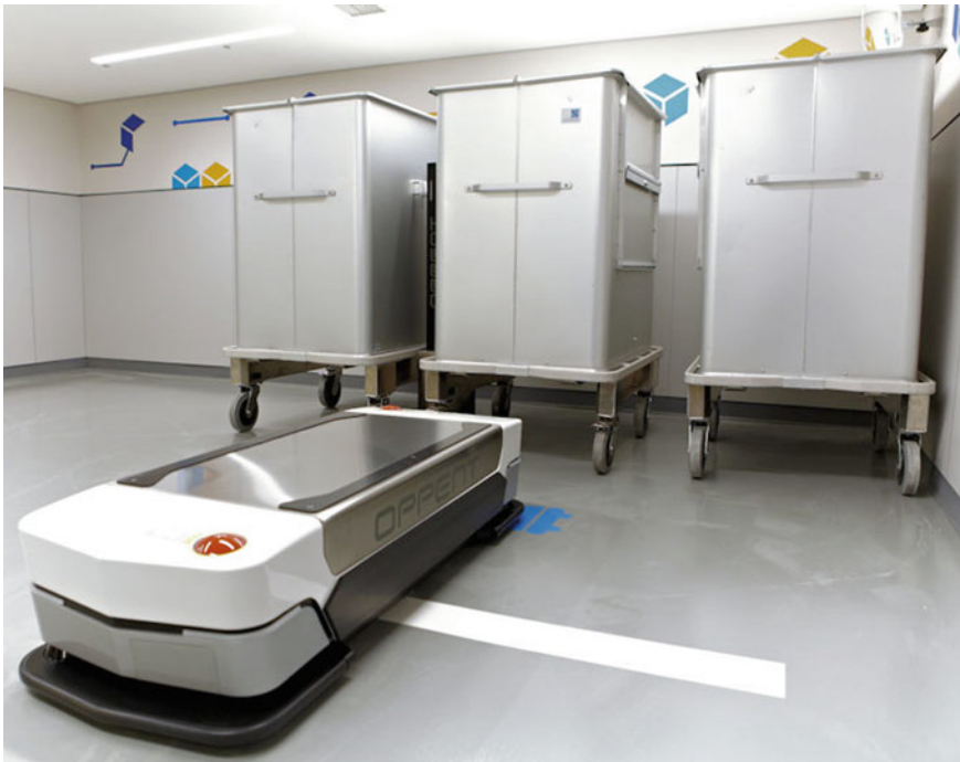
Fig. 7.6 EVOcart™—AGV system at Acibadem Maslak Hospital (Video 6 EVOcart™—AGV system at Acibadem Maslak Hospital [ https://www.youtube.com/watch?v=epeSHuSFNrs ]). Source Oppent.com.tr)
