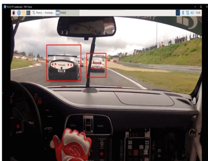
Fig. 5 SSD MobilenetV1 detected vehicles using Raspberry Pi VNC viewer
