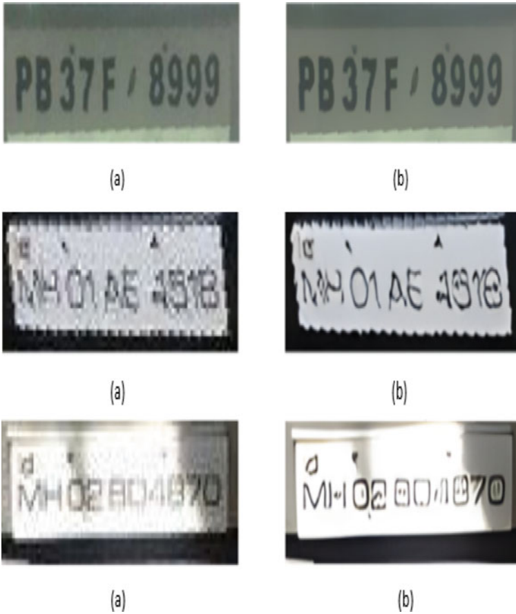
Fig. 6 High quality images by Super-resolution a Input image, b Real-ESRGAN output
