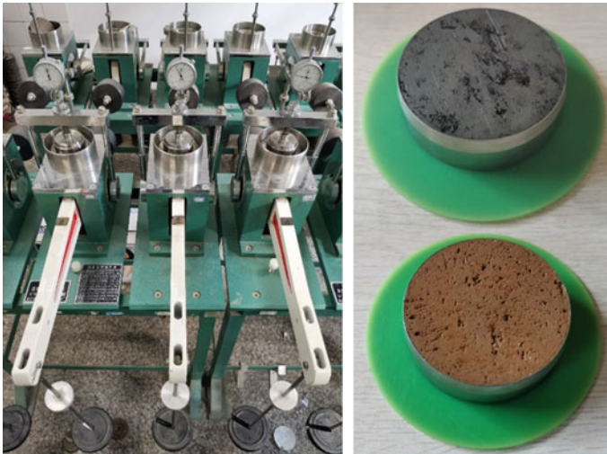
Fig. 1 The consolidation instrument and soil samples
