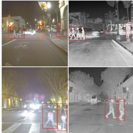
Fig. 1. The pictures in the left/right are captured from the visible/infrared camera. Compared with the pedestrians in the red box of visible picture, the pedestrians in the infrared images are more clear. (Color figure online)
