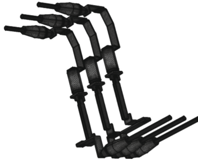
Fig. 2. Busbar and insulator grid sections
