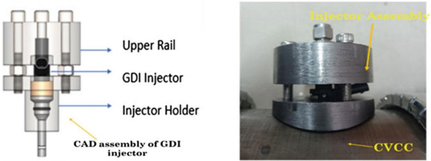
Fig. 11.11 Injector CAD drawing and installation in the CVC
