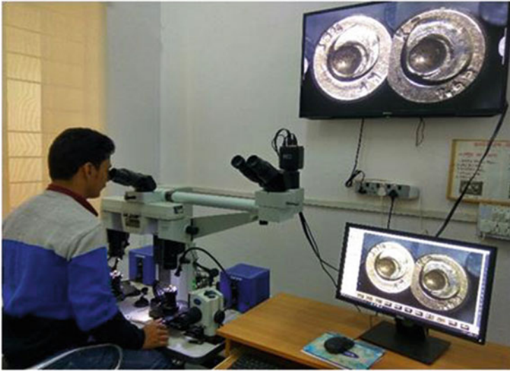
Fig. 15.16 Comparison microscope setup showing comparative matching of firing pin and breech face marks of two cartridge cases in a split view window
