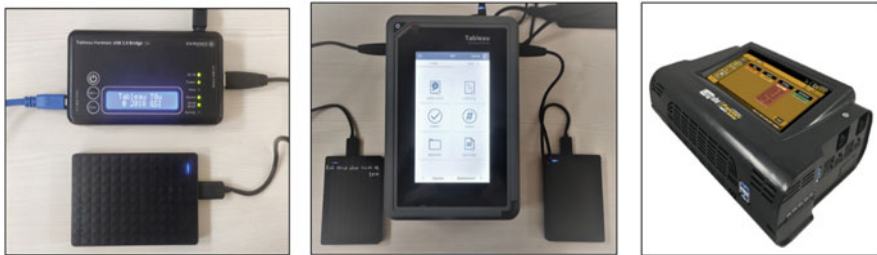
Fig. 25.14 Tableau USB write blocker, Tableau TX1 and Falcon devices (left to right)
