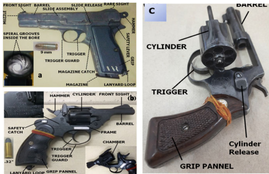
Fig. 15.3 (a) 9 mm semi-automatic pistol (manufactured by RFI India). Inset shows the spiral rifling of right-handed twist inside the bore of the barrel; (b) 0.32" caliber break-top revolver of Indian Ordnance Factories. Lower inset shows the six chambers when the cylinder is open while the upper inset shows the enlarged view of the details in the frame; (c): 0.32" caliber In Swing-out revolver of Smith & Wesson
