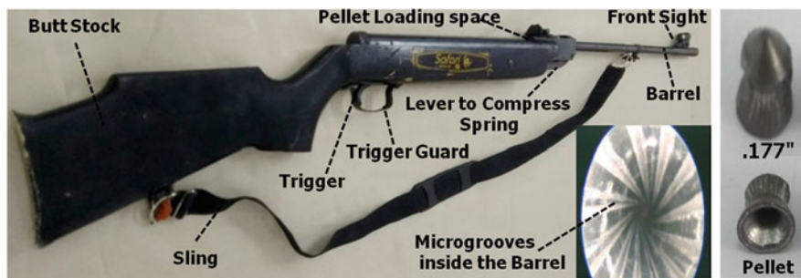
Fig. 15.8 Air rifle of 0.177" caliber along with pellet of 0.177"
