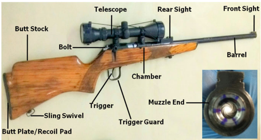
Fig. 15.1 Bolt action rifle of 0.22" caliber. Inset shows the muzzle end and rifling in the bore
