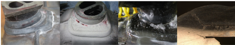
Fig. 9. Leakage test and electron microscope analysis of outer ring crack point
