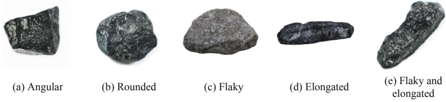
Fig. 2.9 Angularity and flakiness of coarse aggregates
