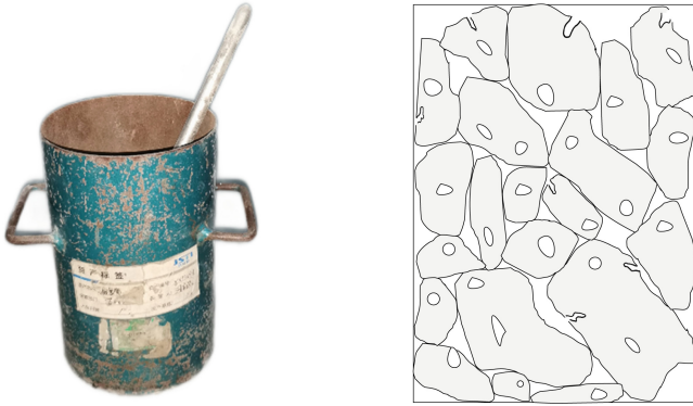
(a) Unit weight test container (b) Aggregates packed in the container
