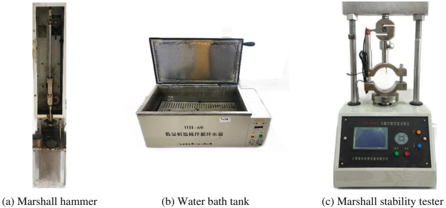
**Fig. 7.9** Marshall stability test apparatus
