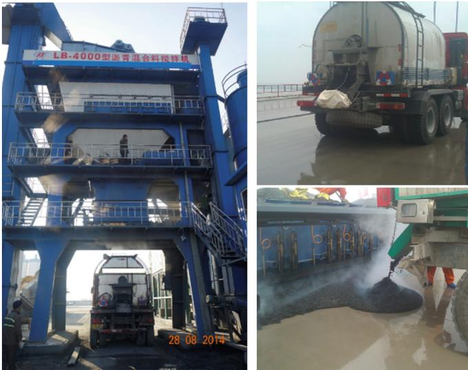
Fig. 7.38 The guss-cooker and paver for gussasphalt
