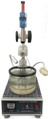
(a) Asphalt penetration tester
