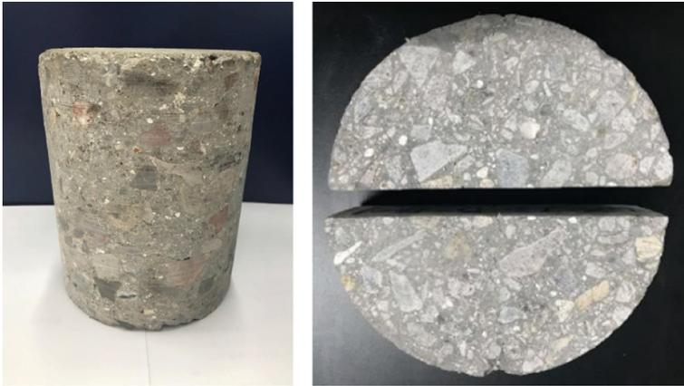
**Fig. 5.1** Cores of cement-stabilized material
