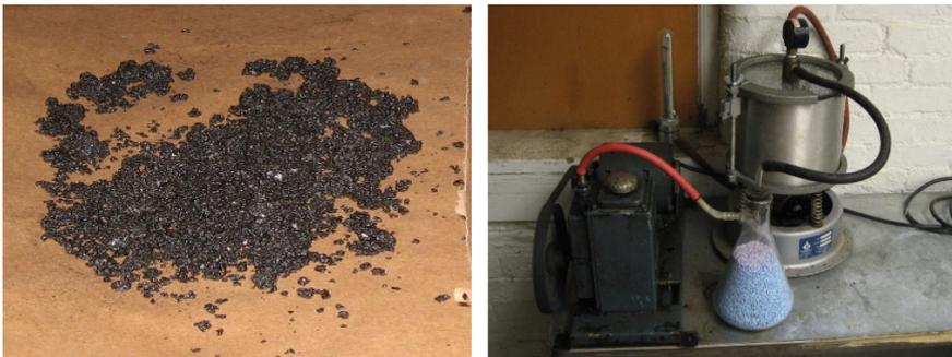
**Fig. 7.32** Theoretical maximum specific gravity test
