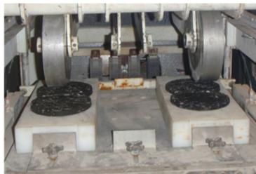
**Fig. 7.12** Asphalt pavement analyzer
