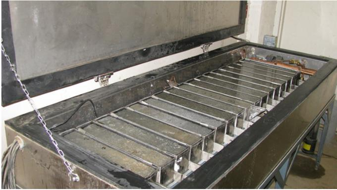
**Fig. 4.27** Concrete rapid freeze–thaw test
