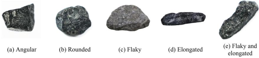
Fig. 2.9 Angularity and flakiness of coarse aggregates
