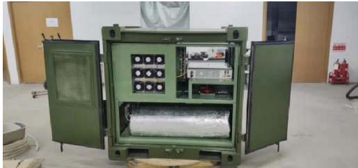
Fig. 4. Methanol reforming to hydrogen fuel cell power supply prototype
