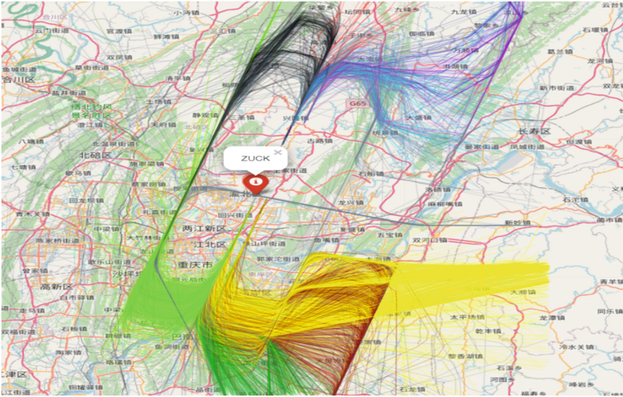
Fig. 2. Spatial clustering results, with different colors representing different air traffic flows.
