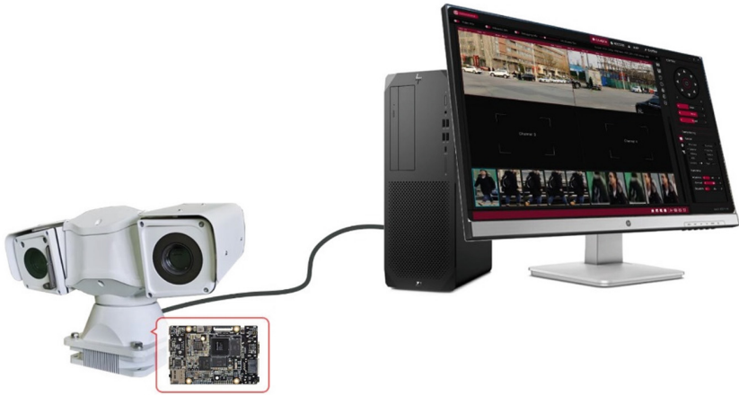
Fig. 6. The Edge-based Implementation of Person Re-identification
