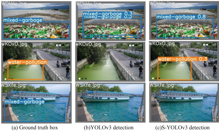
Fig. 4. Example of YOLOv3 and S-YOLOv3 detection
