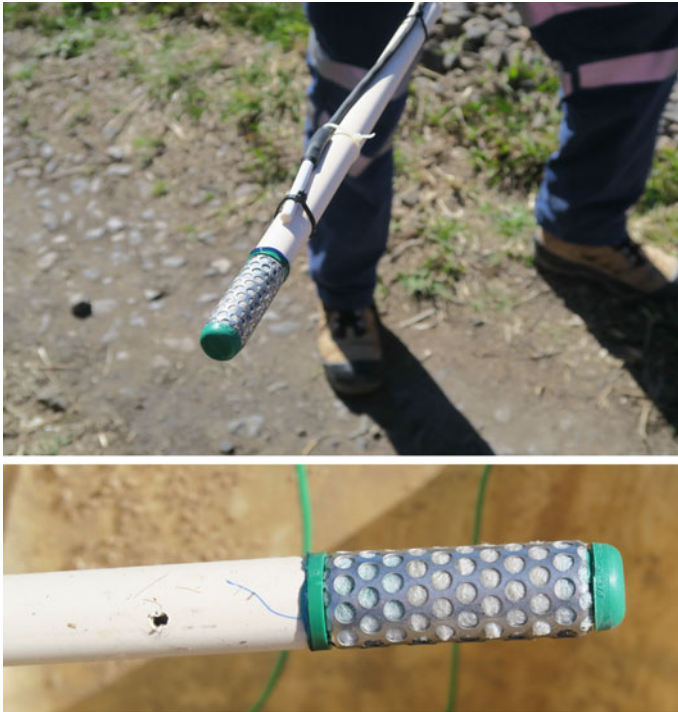
Fig. 3 Watermark 200SS sonde prepared for installation, (top) with temperature monitor attached to outside of PVC conduit in proximity to the sonde and (bottom) the recommended hole in casing just above instrument
