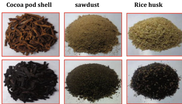
Fig. 2 Comparison of biomass color before and after torrefaction
