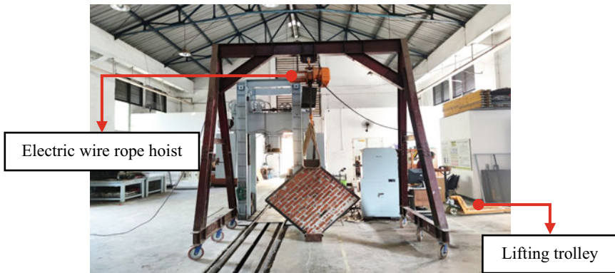
Fig. 3 Mounting of masonry panel into loading frame
