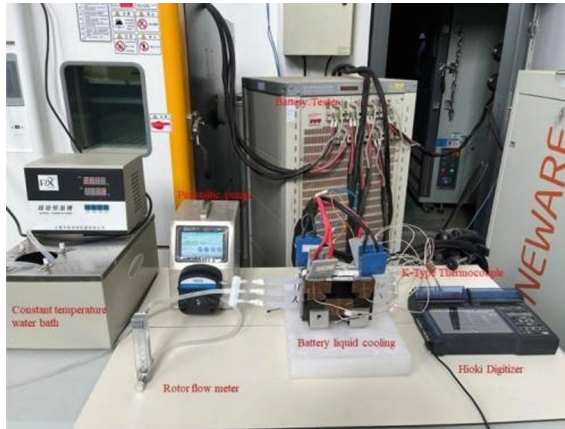
Fig. 5. Battery liquid cooling system experiments.
