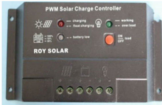
Fig. 3 Solar charge controller or regulator (PWM type)
