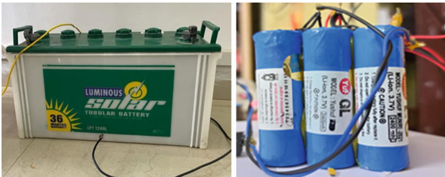
Fig. 4 Solar tubular (12 V 45 Ah) and Li-ion battery (12 V 10 Ah)
