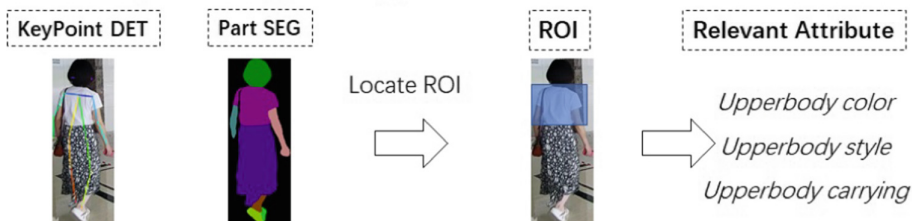
Fig. 5. Relationship of training tasks based on spatial attention mechanism
