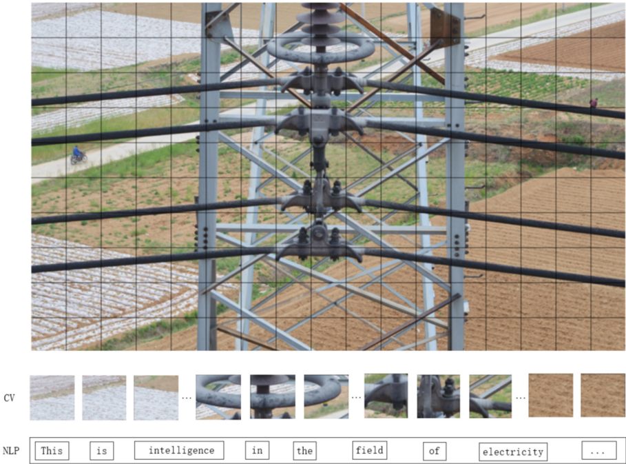
Fig. 2. Image block embedding processing for power transmission pictures, CV is the corresponding image block processing, NLP is word embeddings.
