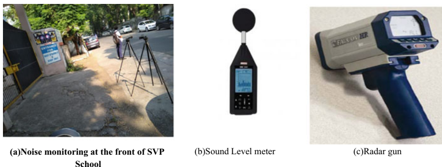
Fig. 1 Photograph of noise monitoring at the front of SVP School (a), Instrument used for noise measurement (b), and vehicle speed measurement gun (c)
