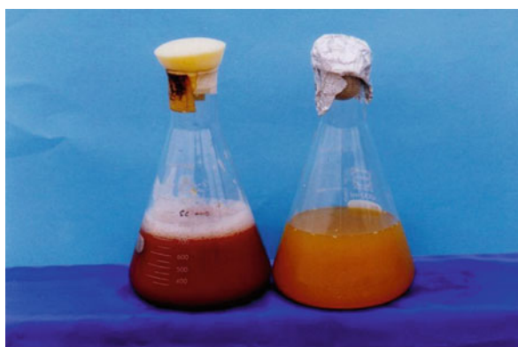
Fig. 15.2 Growth of Rv. sulfidophilum in settled undiluted non-sterilized SPW under anaerobic light with 15% (v/v) of inoculum
