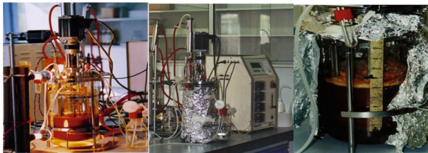
Fig. 15.6 Mass production of Rv. sulfidophilum in SPW with a bioreactor. (Left: in presence of light. Right: dark culture)
