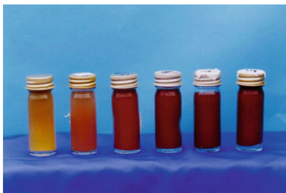
Fig. 15.5 Growth of Rv. sulfidophilum under anaerobic light conditions in non-sterilized settled SPW. (From left to right: Non-sterilized settled SPW without inoculation; Inoculated with Rv. sulfidophilum (0 h); growth after 24 h; growth after 48 h; growth after 72 h; growth after 96 h; growth after 120 h
