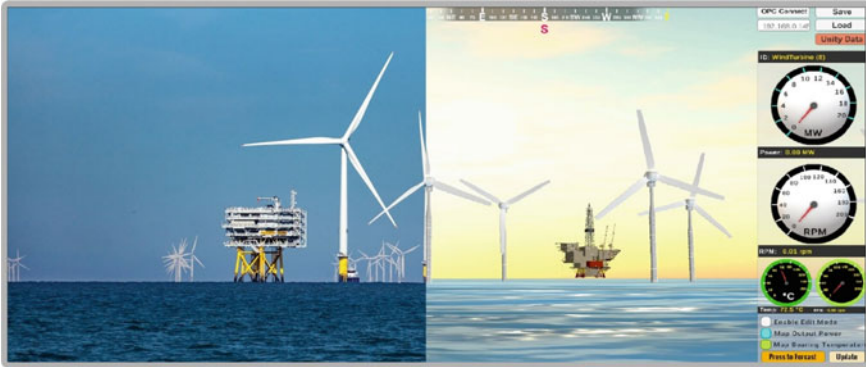
Fig. 2 Wind farm (left) and its digital twin (right)
